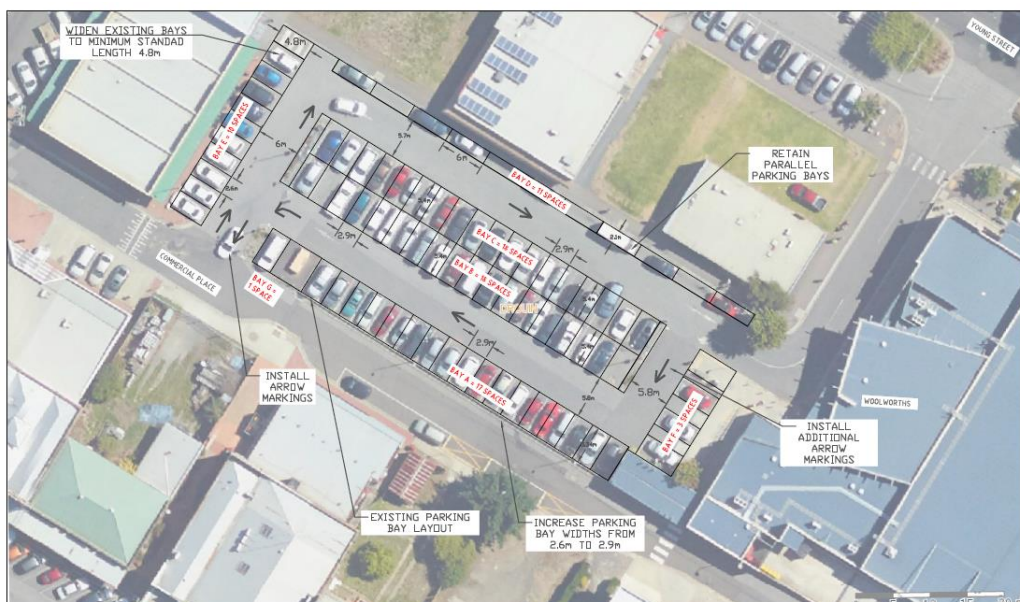
Figure 15 – 90-degree parking configuration option for Drouin Woolworths Carpark
