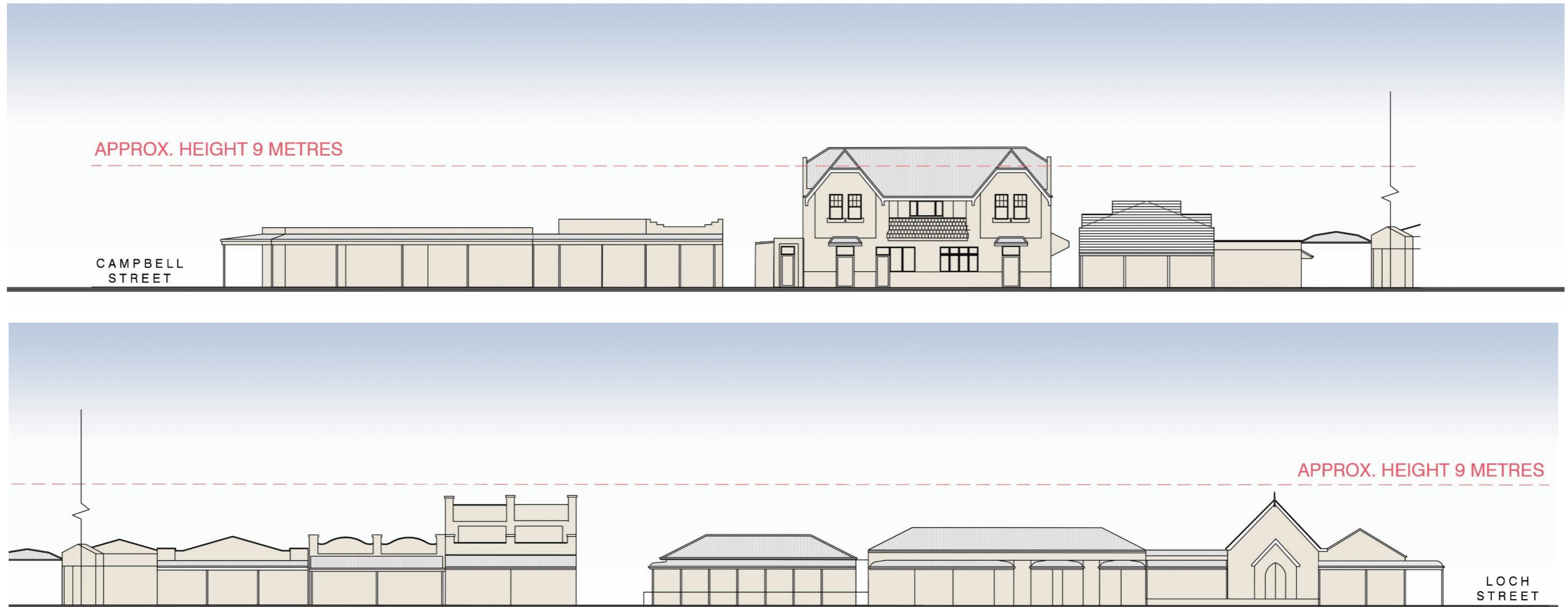
Figure 10: Elevation showing varied roof forms and approximate height of existing buildings on the Princes Highway Service Road between Campbell Street and Loch Street
