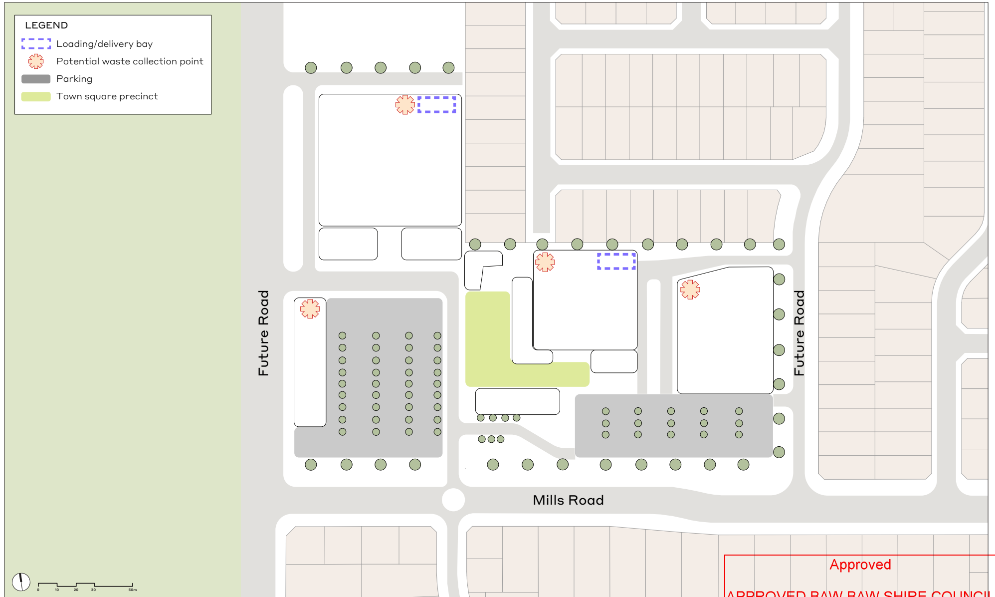
Figure 31. Loading/delivery bays and waste collection
